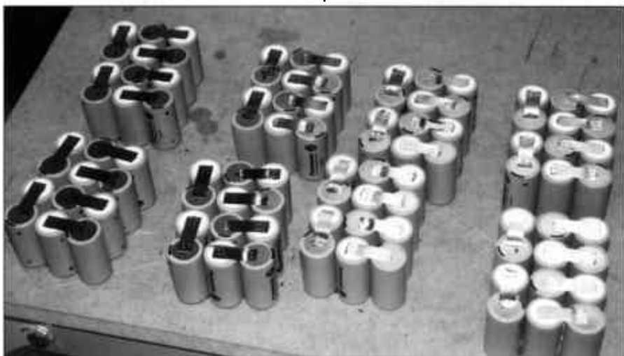
Photo.2: NiCad Batteries in course of production at Akkupak — made up for re-fitting existing cordless tool battery packs
